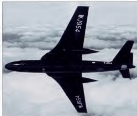
Above: Several B.Mk 1 and B(PR).Mk 1 aircraft were converted to tankers and designated B(K).Mk 1 and BPR(K).Mk 1, respectively.
